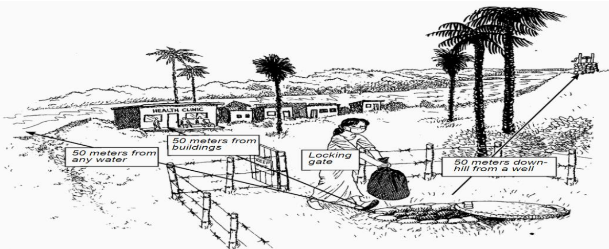
Use the 50 meter rule when you dig a pit to bury wastes.
